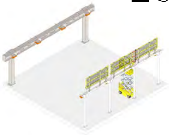
4. Infills are installed between 'goal posts'. This includes a 'cage' at upper floor microcolumn locations, which aids column positioning while maintaining edge protection.
