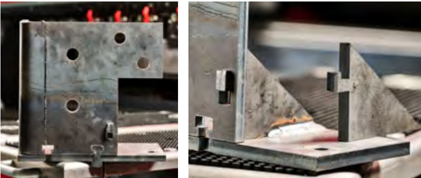
Laser cut Platform II brackets developed by the MTC
