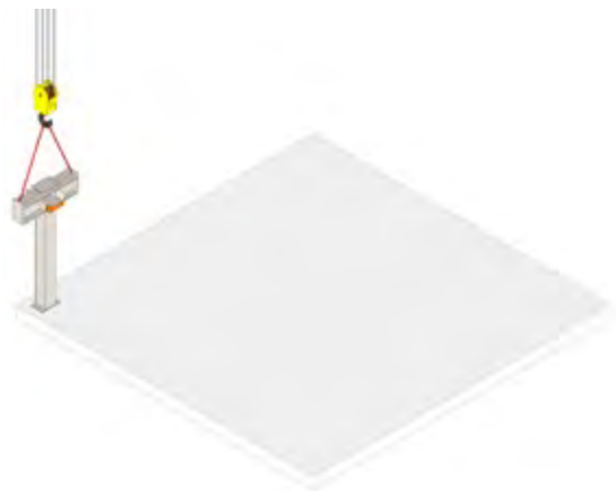
1. Inboard columns are installed using mobile crane. The column head detail is already installed, including fixing brackets for long span beams.
