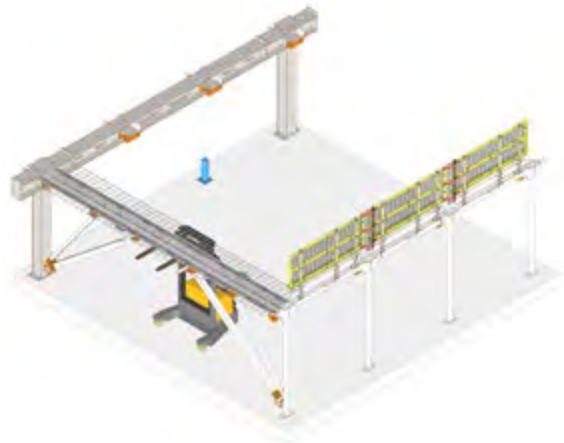
5. Permanent shutters, including rebar cages, are installed using reach stackers. The long-span beams have pre-installed, self-locating 'shoes' into which the shutters drop for accurate positioning. Temporary diagonal props are installed; laser cut components ensure accuracy.
