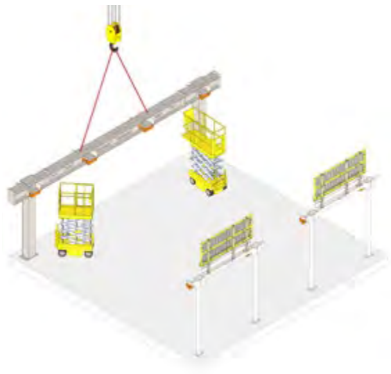
3. Long span-beam is located using a mobile crane. The standard pattern of service provisions and cross-beam fixings are pre-installed. Operatives work in MEWPs to fix the beam to columns using bolted connections to the column heads.
