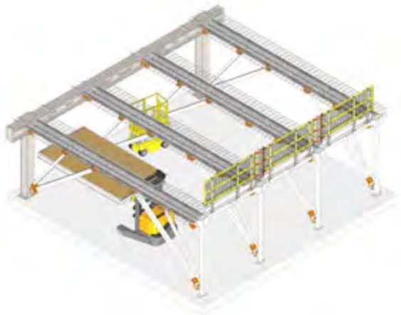
6. Slab shutters are lifted into position using reach stackers. Shutters have reinforcement and fixings for MEP pre-installed before lifting. Reinforcement links are installed from a Mobile Elevated Work Platform (MEWP).
